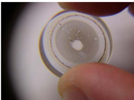
Fig. 8: Ablation: Nd:YAG laser, 5 ns, 10 mJ
