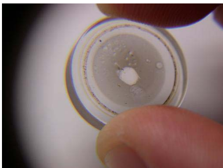
Fig. 8: Ablation: Nd:YAG laser, 5 ns, 10 mJ
